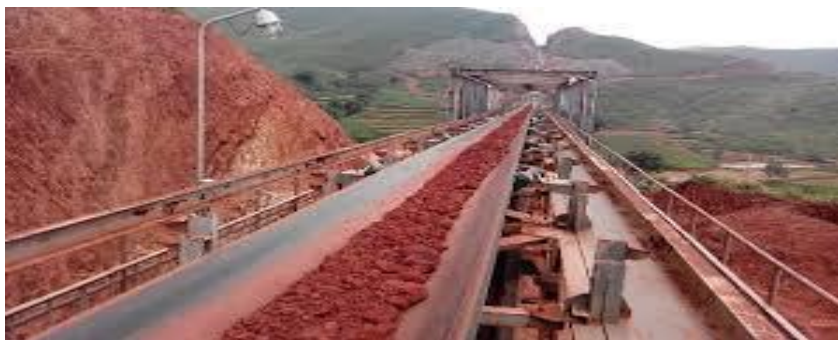
Fig 75 – ~18km conveyor belt from Baphimali mine to Utkal
